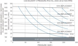
C38 DELIVERY V PRESSURE (POLYOL, 2000 cSt @ 1500 RPM)
