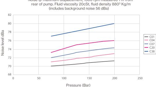
Noise @ maximum displacement, 1500 rpm measured 1 m from
